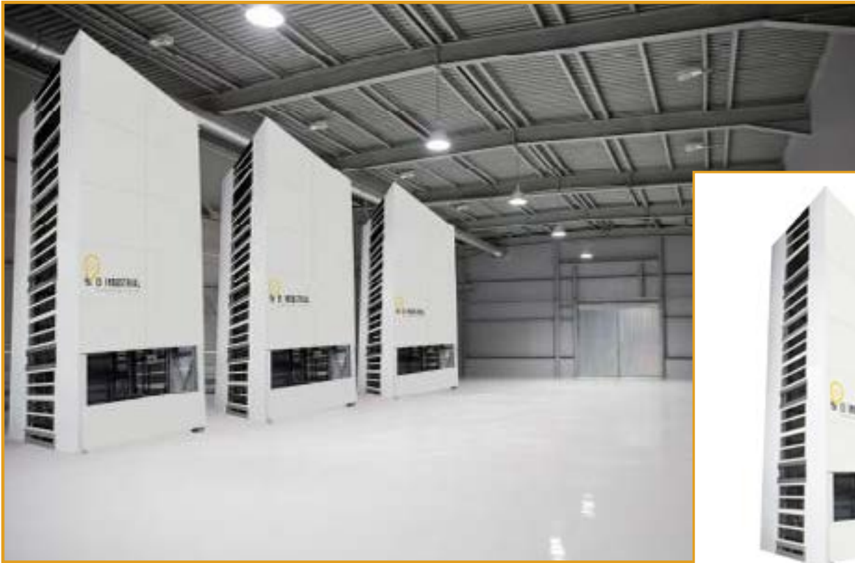
EI Vertical, one of the products from EI Automation, is an automated vertical warehouse system that helps factories save space, cost, and labor force as well as increase productivity, traceability, and security. Photo credit: EI Automation
